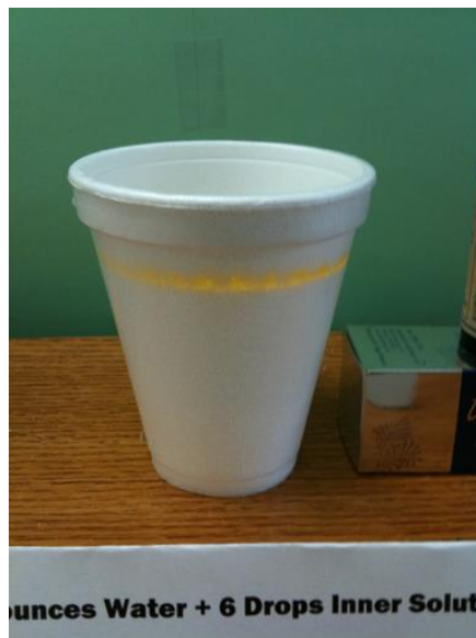
Melted through cup walls at 2 min 24 sec
